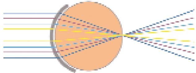
Illustration 2. Changing the curves of the lens surface enables light rays to converge to a single point.
