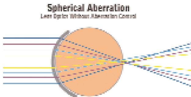
Illustration 1. Lens design induces spherical aberrations causing light rays to strike the retina in multiple focal points.
