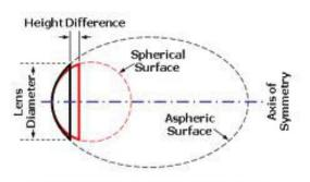
Aspheric Versus Spherical Surface
